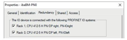
Apply this hardware configuration to operate *ibaBM-PN* in the S2 redundancy mode.
